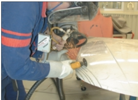
Simultaneous monitoring of isocyanates using impinger-filter sampling and a continuous monitoring device.
