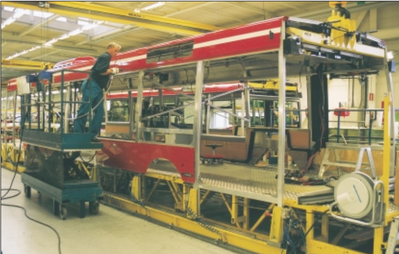
Windows are mounted using a non-isocyanates containing glue.
