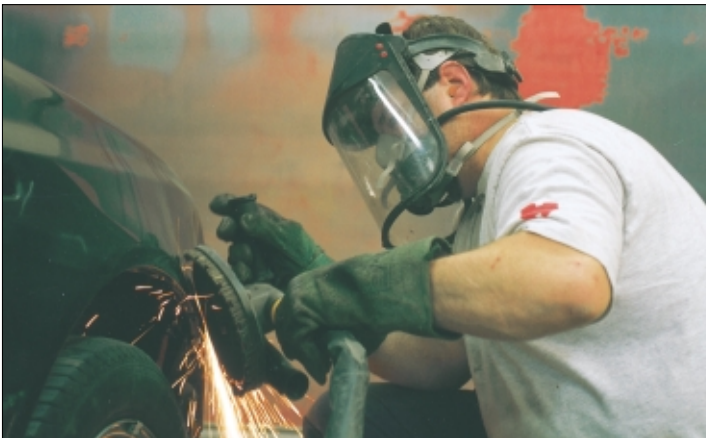
The use of fresh air respiratory protection device during grinding.
