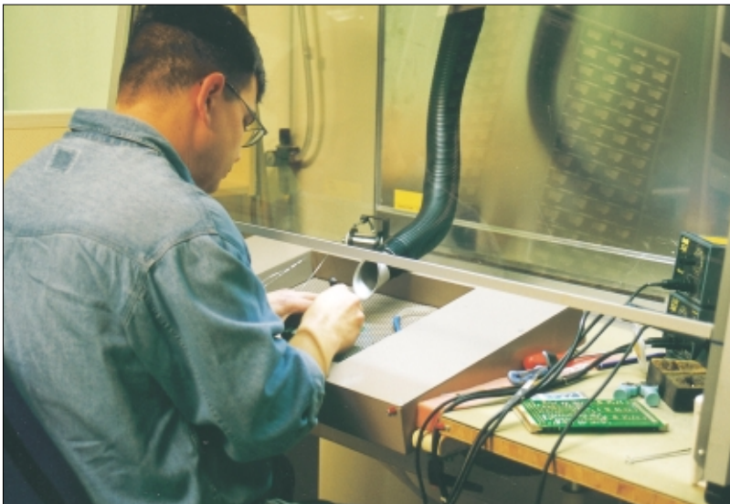
Soldering of a PUR lacquer circuit board.
